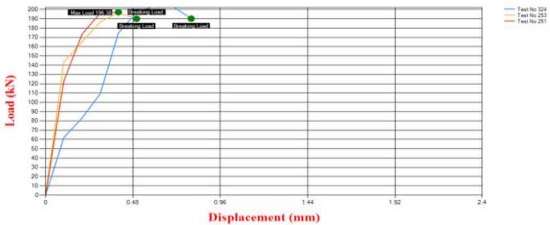
Figure.6.Graph showing the Load-Displacement variation of cube using low density aggregates (After 14 days moist curing)
