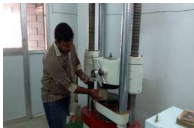
Figure.3. Compression test in the UTM
