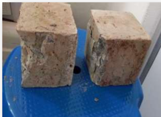
Figure .9. Cubes after compression test
