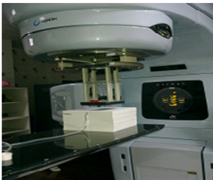
Figure 1.a: Measurement set up with LINAC along with plastic water phantom
