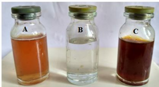
Figure .2 Visual observations (A) Plant extract (B) Copper chloride solution and (C) formation of CuO NPs
