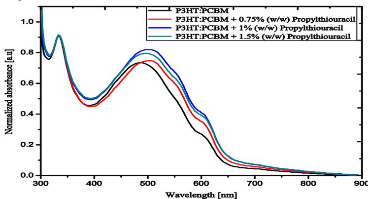
Figure. 3 Normalized absorbance of thin films of P3HT:PCBM with different concentrations of PTU
