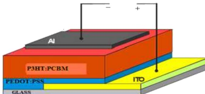
Figure. 2 Basic device structure of bulk heterojunction solar cell used in this study
