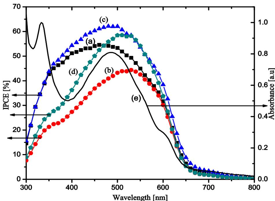
**Figure. 8 IPCE spectra of P3HT:PCBM (a) without PTU (b) with 0.75% (w/w) PTU (c) with 1% (w/w) PTU (d) with 1.5% (w/w) PTU (e) absorption spectra of P3HT:PCBM.**
