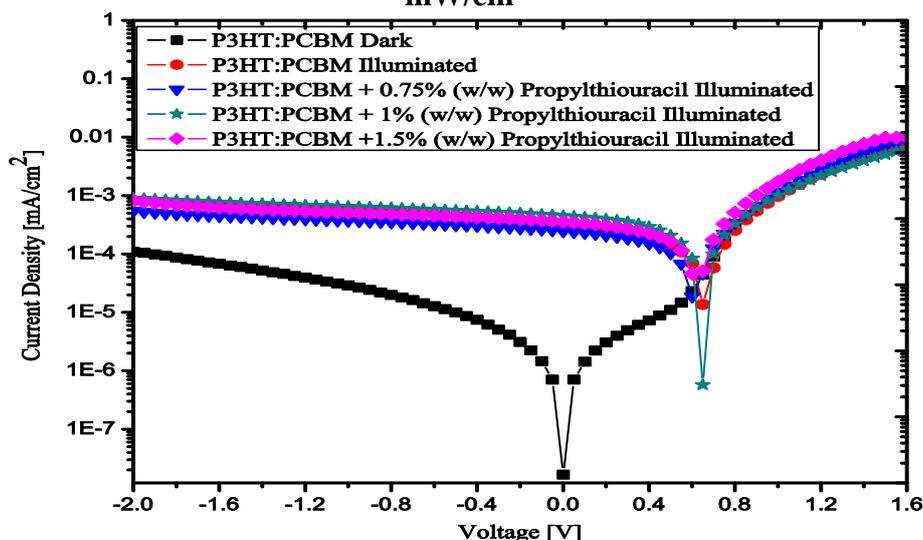
**Figure. 6** Semi-logarithmic J-V characteristics of P3HT:PCBM with different concentrations of PTU additives in the dark and under white light illumination with incident light intensity of 80  $\text{mW}/\text{cm}^2$
