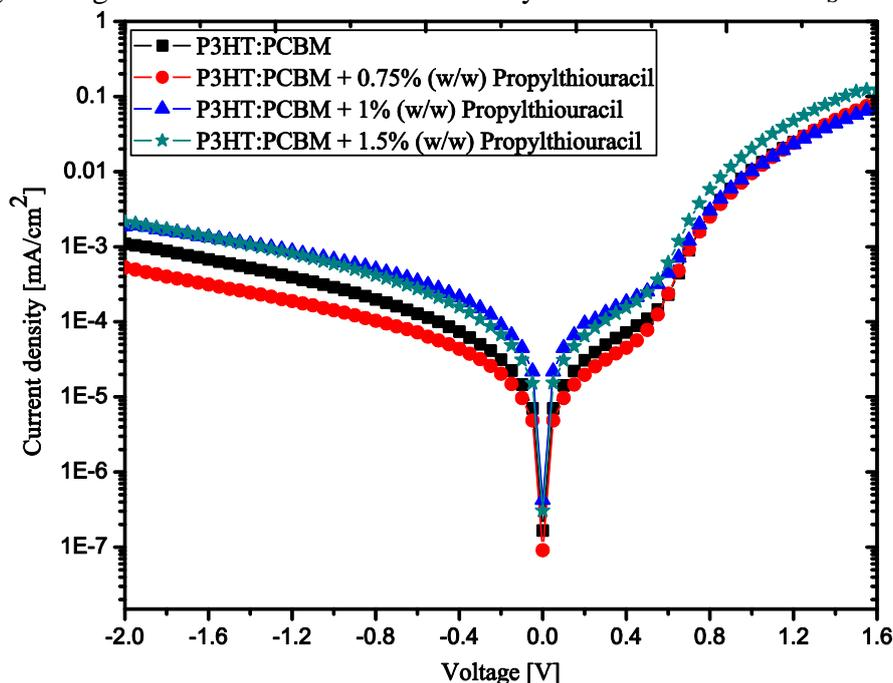
**Figure. 4** Semi-logarithmic dark current density-voltage characteristics of P3HT:PCBM with different concentrations of PTU
