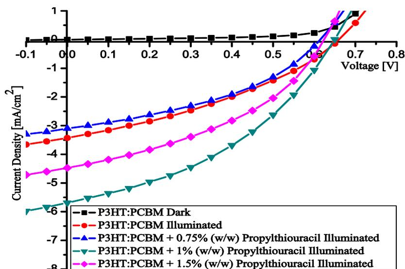
**Figure. 5** The J-V characteristics of P3HT:PCBM with different concentrations of PTU additives in the dark and under white light illumination with incident light intensity of 80  $\text{mW}/\text{cm}^2$
