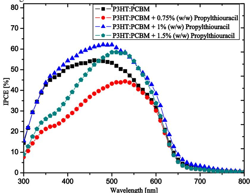
**Figure. 7 IPCE spectra of P3HT:PCBM with different concentrations of PTU additives**
