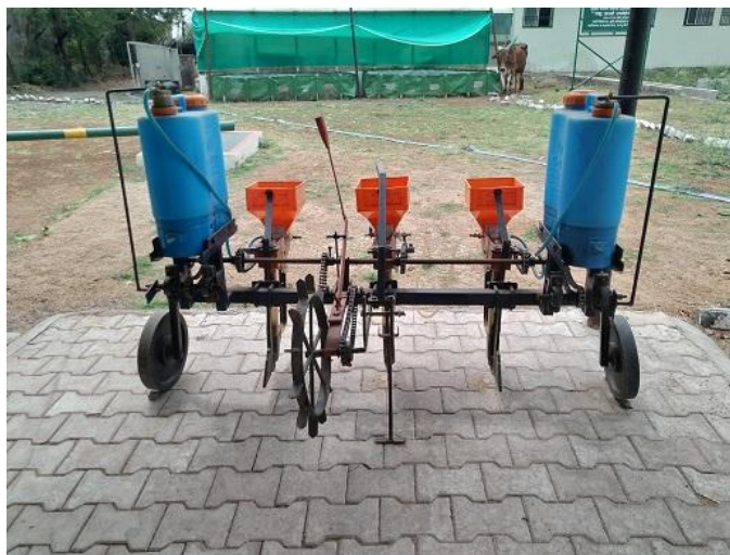
Fig. 1 : View of developed three row animal drawn multi crop planter cum herbicide applicator
